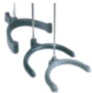
BASE A FERRO DI CAVALLO IN GHISA 150 mm C/ASTA Ø 10x500 mm IN ACCIAIO
