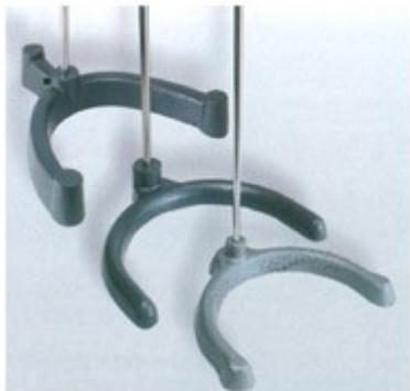
BASE A FERRO DI CAVALLO IN GHISA 225 mm C/ASTA Ø 12×600 mm IN ACCIAIO
